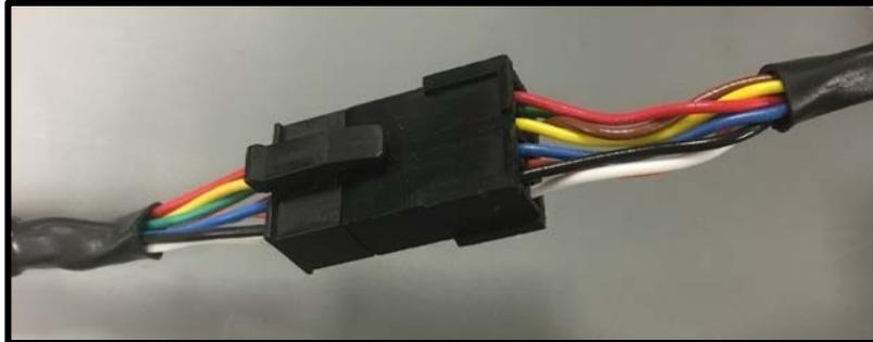
*Figure 11 Check connector and wiring between JX VEHICLE MODULE and TX55*
