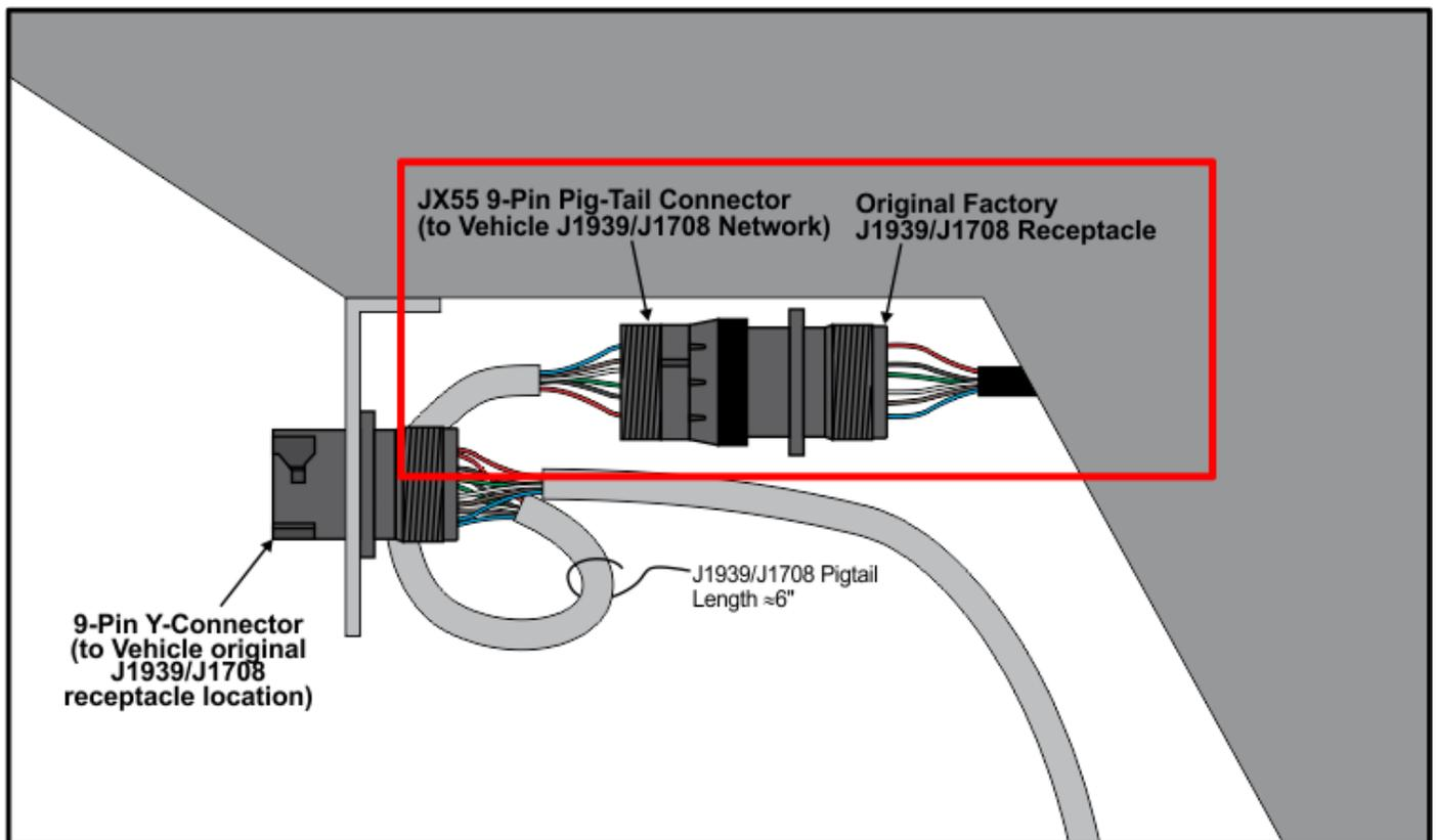
Figure 3: Typical Y-harness connection to bus
