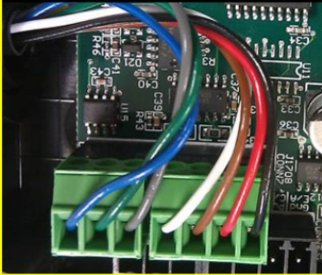
Ensure the colored wires that are in the green plugs on the circuit board from Right to Left are in the correct order. This is the pin config for J1939 termination inside the JX55 Box
