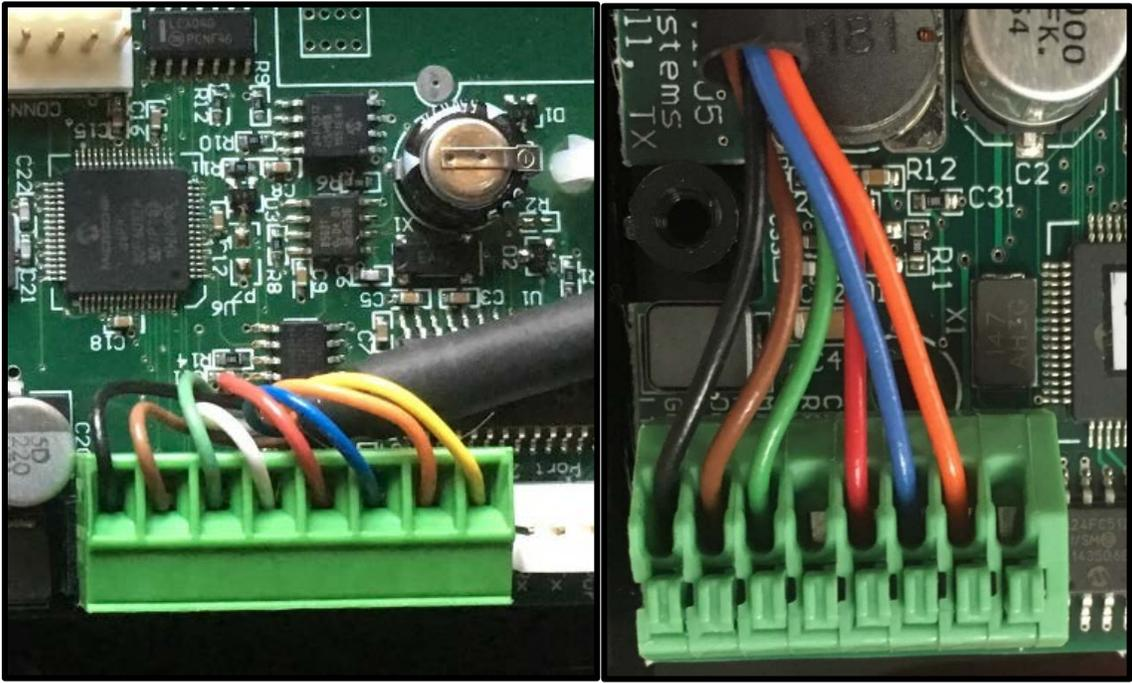
*Figure 9: On left, TX55 connector inside JX VEHICLE MODULE and on right, wiring from JX VEHICLE MODULE inside the TX55.*
