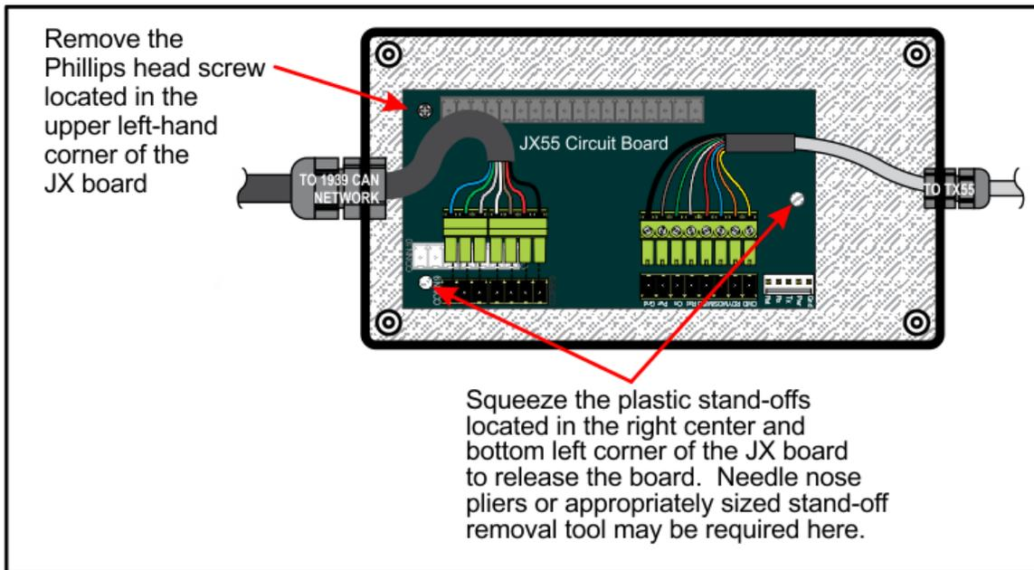
**Figure 16: Remove mounting screw and release board from stand-offs**
