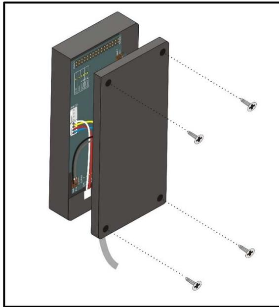
*Figure 14: Remove lid to access inside JX VEHICLE MODULE data logger*
