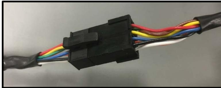
*Figure 5: Connector plugged in between JX VEHICLE MODULE and TX55, normal operating mode*
