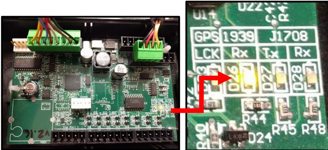
**Figure 7: LED lit when JX VEHICLE MODULE receiving power from bus**
