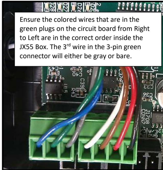
**Figure 10: JX VEHICLE MODULE power and data lines inside JX VEHICLE MODULE box.**
