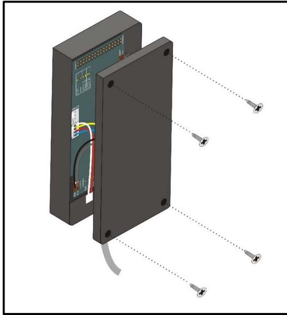
**Figure 6: Remove lid to access inside JX VEHICLE MODULE data logger**
