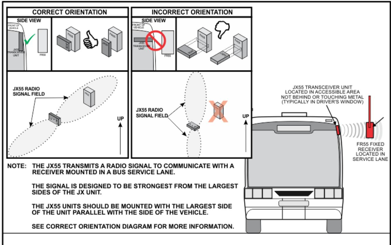
Figure 12: Note proper placement of TX55. Avoid installing TX55 on metal surfaces. TX55 must pass FR55 receiver in fuel lane. Proper placement required.
