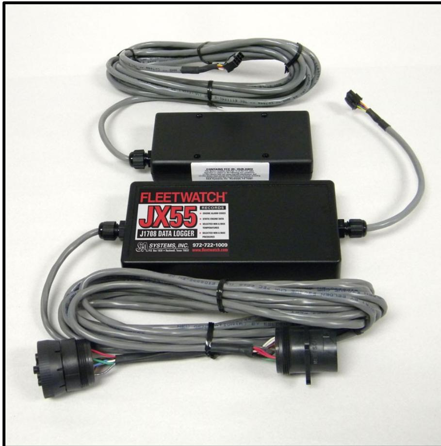
JX VEHICLE MODULE with Y-harness and TX55 Transmitter
