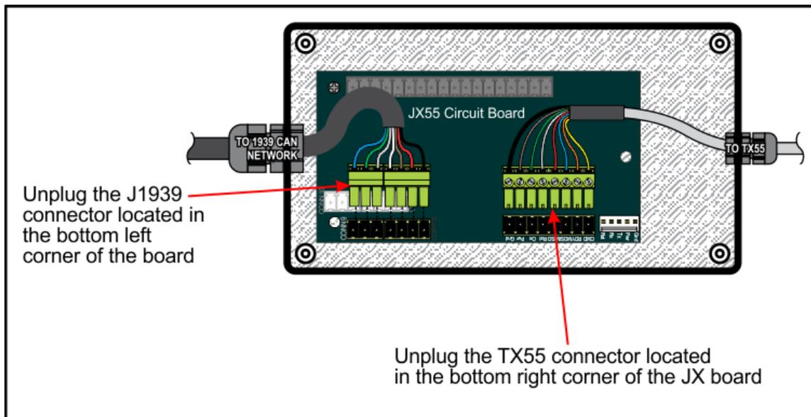
*Figure 15: Remove J1939 and TX55 connectors*
