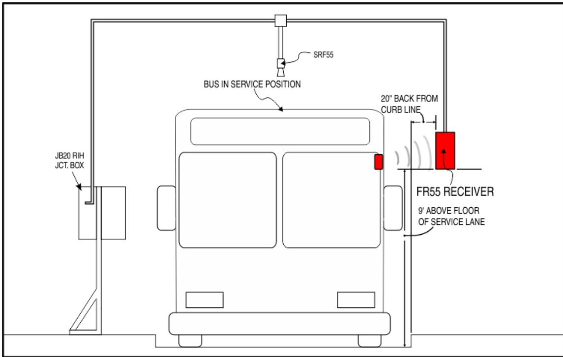
Figure 13: Ensure the module doesn't stop short of the FR55 receiver.
