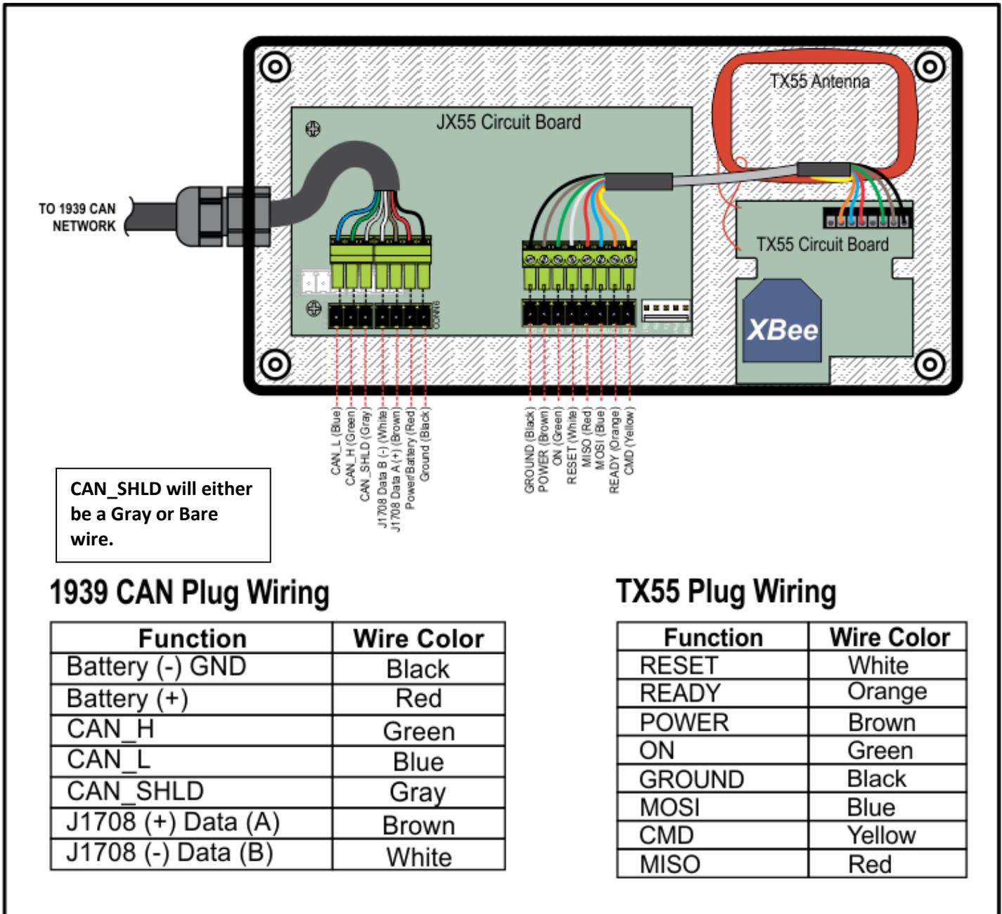
Figure 2: Overview schematic of JX VEHICLE MODULE-1939
