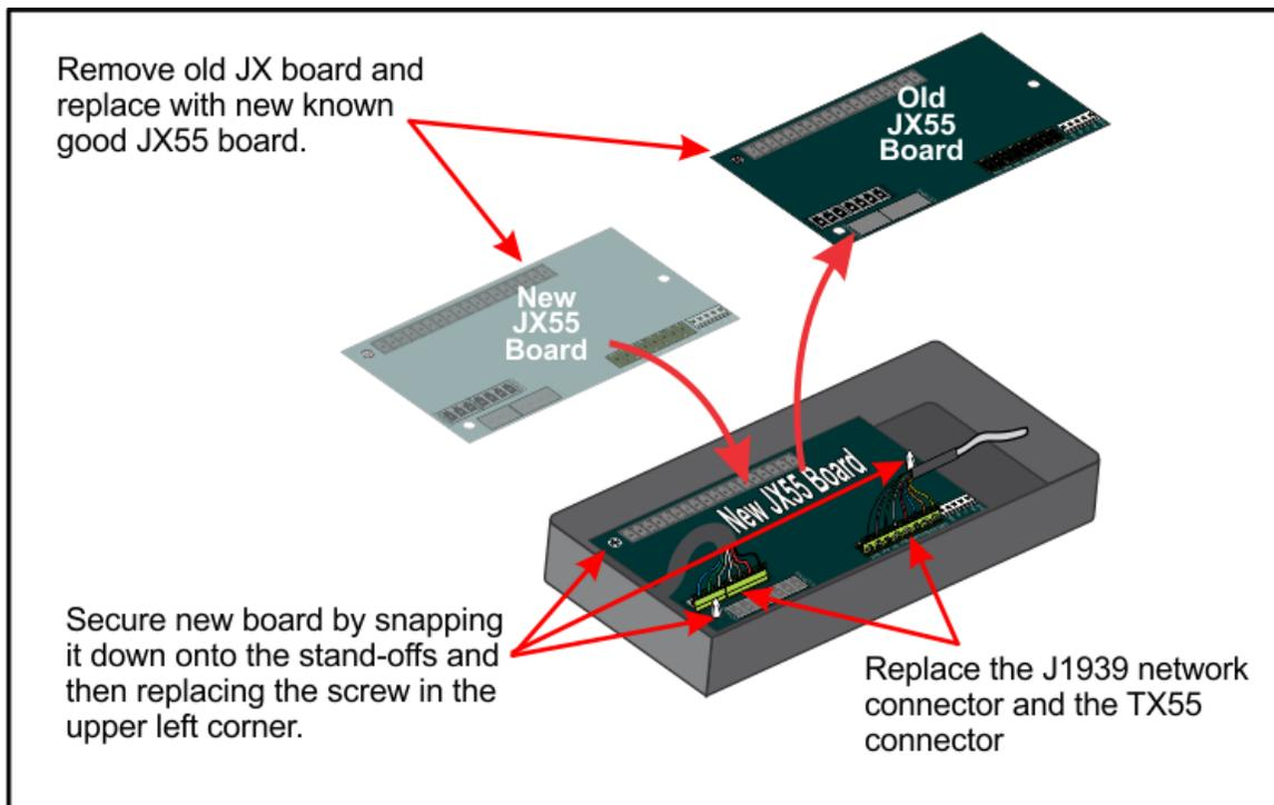
**Figure 17: Replace JX board, secure, and reconnect**
